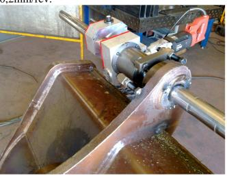
Optional: Facing attachment to machine thrust faces.
